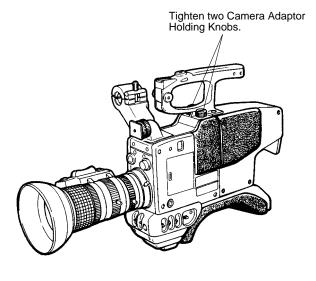
2-2 Remove the Camera Adaptor while pressing up the Release Button underneath the camera.
